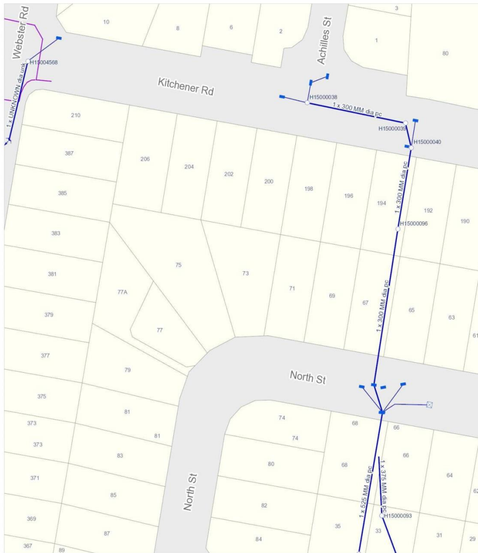
BCC Stormwater and Cable Networks
